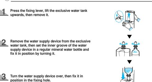
Turn the water supply device over, then fix it in position in the fixing hole.
