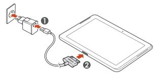
Connecting the USB cable improperly may cause serious damage to the device or USB power adapter. Any damage caused by misuse is not covered by the warranty.
