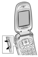
In Idle mode, you can also adjust the keypad tone volume using these keys.
