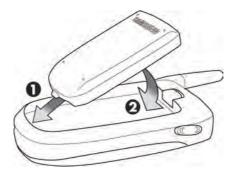
Gently push the top end of the battery down (The top end of the battery displays the word Samsung in raised letters.) until you hear it click into place.
