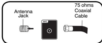
For basic Cable TV service not requiring a Converter/Descrambler box, connect the 75 ohms Coaxial Cable directly to the Antenna Jack on the back of the TV.
