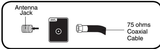
Connect the 75 ohms cable from the combination VHF/UHF antenna to the Antenna Jack.
