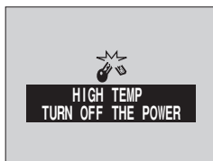
<High Temperature Warning Screen>
