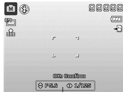
Displays the aperture and shutter speed value
