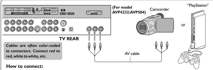
Connect the Audio/Video cables between the Audio (L/R)/Video jacks on the unit and camcorder.
