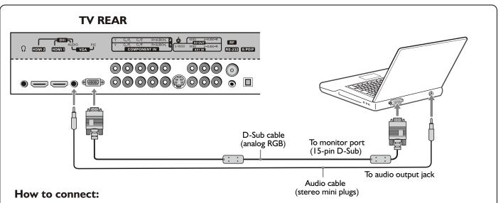
Connect a VGA cable between the VGA jack on the computer and the VGA input jack on the unit.
