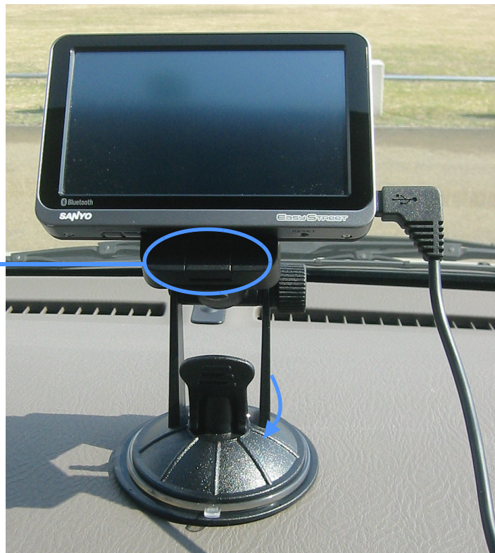
Figure 8: Mounting on the dashboard
