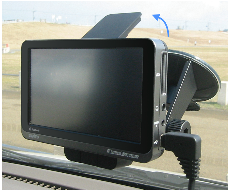
Figure 6: Mounting on the windshield
