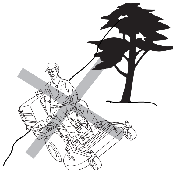
Figure 4-8 Improper Operation on a Slope
