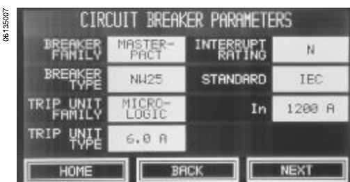
Figure 64: Circuit Breaker Parameters Screen
