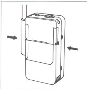
Fig. 6: Attaching the clip
