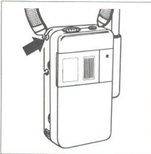
Fig. 5: Attaching the strap
