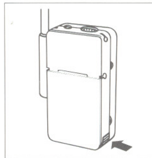
Fig. 1: Opening the battery compartment cover
