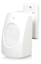
The sensor has a 110° field of view horizontally, and a slightly narrower view (approximately 70°) vertically. This means that most of what you could see if you closed one eye and put your head where you'd mount the sensor is pretty close to the area the sensor will cover. The main blind spots, of course, are above, below or behind the sensor itself.
