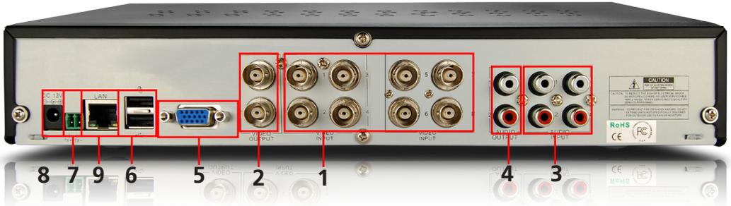
**1) CH1 ~ CH8 (Video Inputs):** These are the eight camera inputs, labelled as per their channel in the DVR's interface. Thus, plug the camera you want to be associated with Channel 1 into the port marked CH1 and so on.
