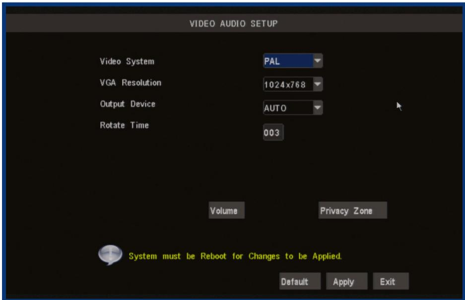
**Video System:** Here you can choose between PAL and NTSC. PAL is used in Western Europe and Australia, NTSC is used in the US, Canada and Japan. If the DVR's picture is black and white, flickering or similar, then this is probably caused by the video system being set incorrectly.
