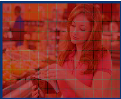
In this example, the entire screen area is activated. A sufficient amount of movement (depending on your sensitivity settings) anywhere in the screen will trigger the motion detection.
