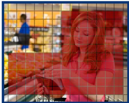
This example shows the same image, but the top left side of the motion area is not activated, and neither are the edges of the screen. Movement in these areas will not trigger the motion detection.
