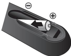
Make sure to match + and - on the batteries to the marks indicated in the battery compartment.
