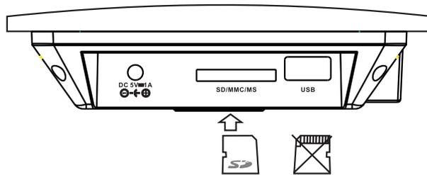
**Note: Please don't disconnect USB device or plug out SD/MMC/MS card while they are working with the unit. Function failure may occur in case of wrong operations.**
