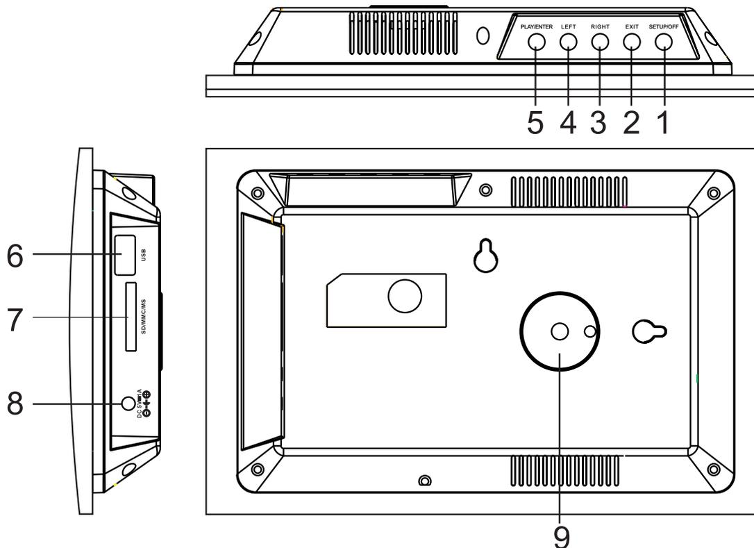
1. **SETUP/OFF:** Power on, Press exit key then press set up button enter into Menu. / Press long (above 2 seconds) to power on and off.
