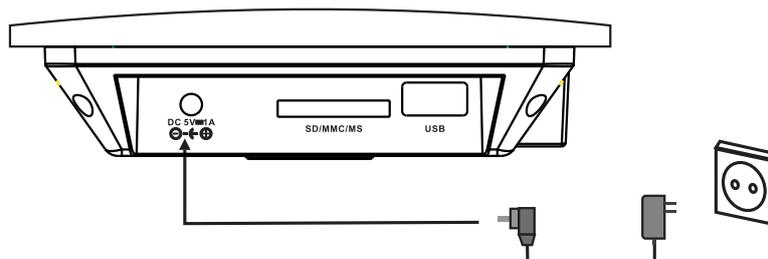
Plug one end of the supplied AC power adapter into the DC input jack of the unit, then plug the other end into the AC power receptacle. Please refer to the illustration above.
