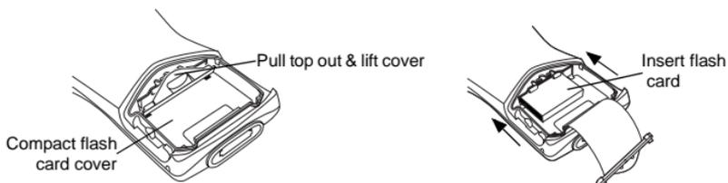
4. To fit the card into place, push down and in at the same time, so that the lip of the compact flash card slips *under* the tabs of the locking mechanism.
