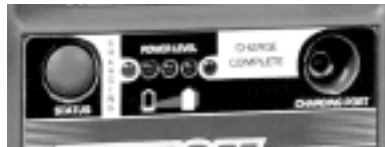
Figure 2. Test Button, Charging, Power Levels and Charge Complete LEDs
