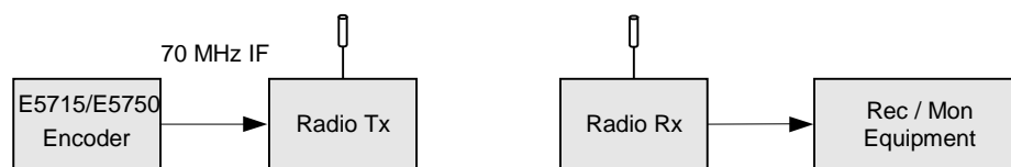
Figure 1.6: Typical DENG System Configuration
