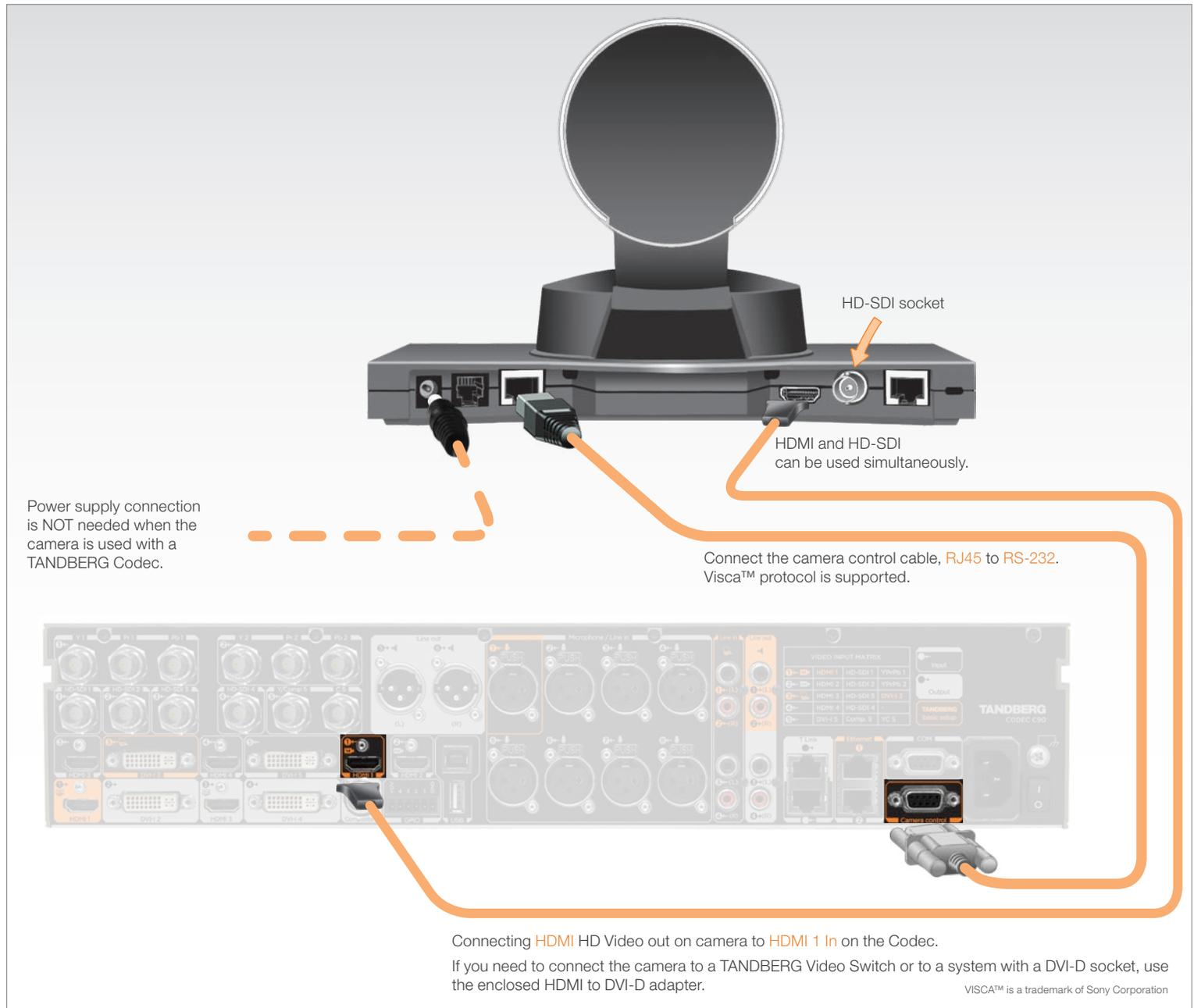
Power supply connection is NOT needed when the camera is used with a TANDBERG Codec.
