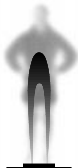
Tanita's patented "foot-pad" design sends a safe, low-level electrical signal through the body to determine its composition.
