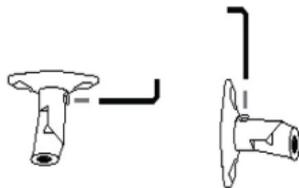
Tighten the allen screw using the provided allen wrench.
