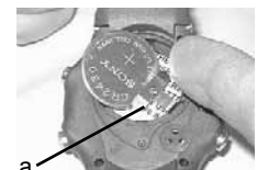
Fig. 117 - AMPHOS BATTERY REMOVAL
