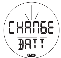
Fig. 4 - LOW BATTERY ALARM
