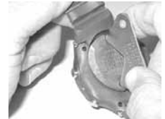
Fig. 120 - BATTERY COVER INSTALLATION
