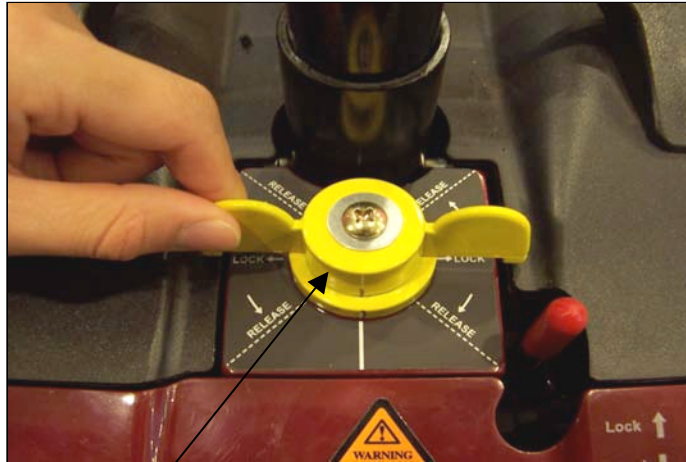
Battery pack lock lever (in the locked position)
