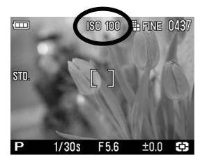
The photosensitivity of digital cameras is described in terms of "ISO equivalent" like silver-halide film cameras. (ISO sensitivity **P.112**)
