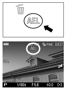
Center the subject, for which you wish to lock the exposure, inside the color LCD monitor and press the AEL button.
