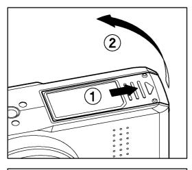
Make sure the camera is turned off and open the Battery / Card Cover in the direction as shown by the arrow.
