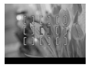
The DP2 is equipped with 9 focusing points and it is possible to select the desired focusing point.
