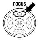
When setting AF mode to normal autofocus (without an icon), the focusing distance is from 28cm to infinity. It is possible to change AF mode to LIMIT mode ( $\underline{\bullet}$  is displayed) by pressing the **FOCUS** button. In LIMIT mode, the focusing distance will be from 1m to infinity and the AF speed will be faster.
