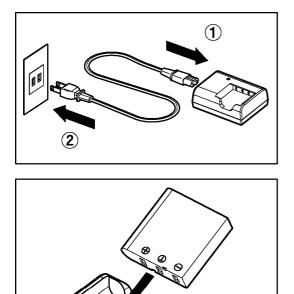
Connect the power cable to the charger and insert the plug into the wall outlet.
