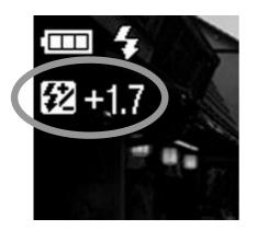
Press the W button after ejecting the flash by using the Flash Pop-up lever. (The Allocate function guide will be displayed on the bottom of the LCD monitor. The 22 icon and the orange compensation value will be displayed in the upper-left corner of the LCD.)
