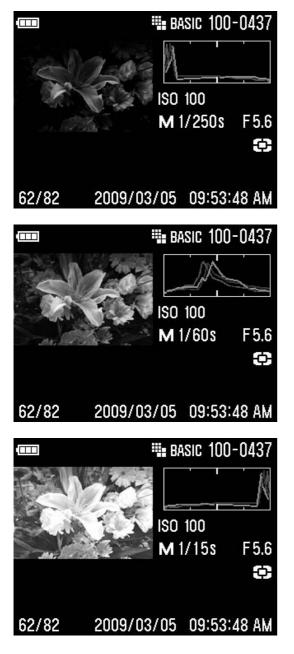
This histogram shows that the higher pixel values are never used in the image, indicating that the image is underexposed, and therefore will appear dark. In general, when the histogram is higher on the left side, the image is mostly composed of dark pixels, causing it to appear dark—either because the image is underexposed or because it is a dark scene such as night shot or sunset.
