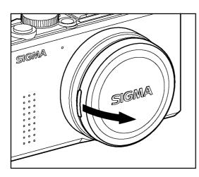
Remove the lens cap as shown.
