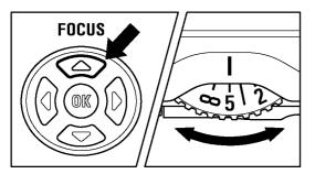
In situations where autofocus or focus lock is not effective, you can focus manually.
