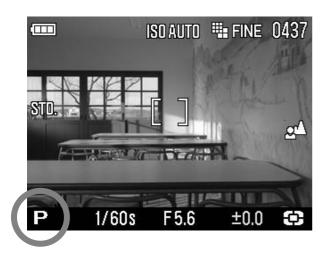
Set the Mode Dial to the **P** position. (The exposure indicator is illuminated in green.)
