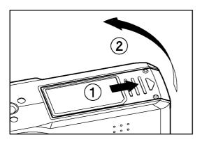
Turn off the camera and open the Battery/ Card Cover, as shown in the illustration.
