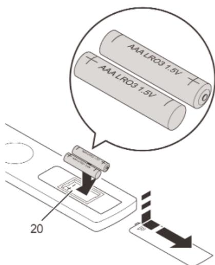
1. Open the battery compartment (20) in the direction indicated by the arrow.
