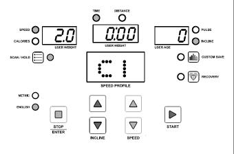
When the computer is in save program status, the "CUSTOM SAVE" button will blink slowly. Press the button to save this program or press the STOP/ENTER button to delete the program and return to POWER ON status.
