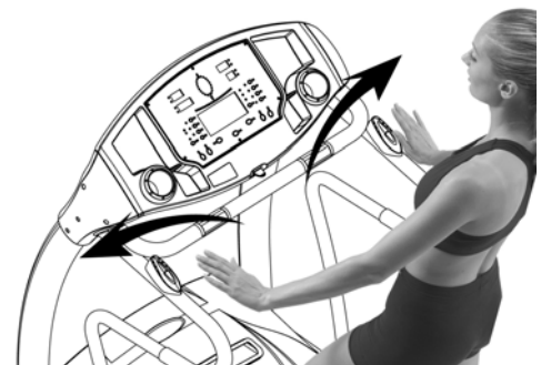
4. Use both sensors to stop belt.
