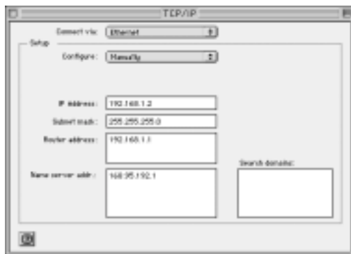
Figure 25. Manual Configuration of IP Addresses
