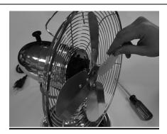
5) Slide the fan blade onto the mounting shaft with the shaft sleeve facing the motor. Align securing screw with flat groove in the motor shaft and tighten with Phillips screwdriver.
