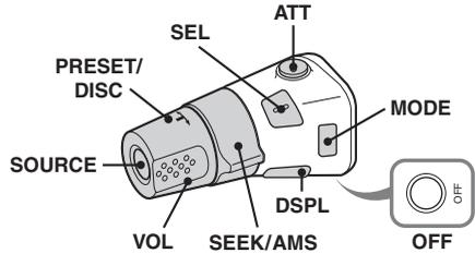
The following controls on the rotary commander require a different operation from the unit.
