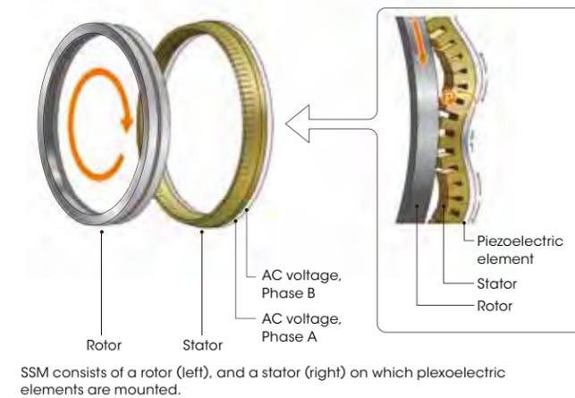
SSM consists of a rotor (left), and a stator (right) on which piezoelectric elements are mounted.
