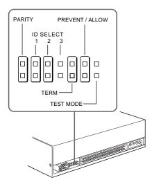
Removing the jumper from a jumper pin pair disables its corresponding function, and installing the jumper enables it. The recommended jumper for use is AMP Shunts (14227-1), JAE Short Socket (PS-2SH4-1) or equivalent.
