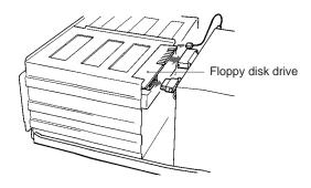
Remove the floppy disk drive and the blanking plate.
