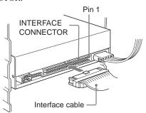
**2** Attach the other end of the cable to the host adapter.
