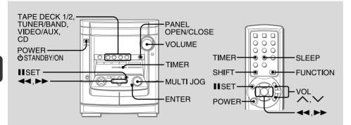
\* Open the control panel with PANEL OPEN/CLOSE if needed.
