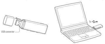
When the remaining battery indication of the display shows: **Full**, charging is complete. When you use the player for the first time, or if you have not used the player for a long time, recharge it fully until **Full** appears on the screen. Charging takes about 60 minutes when the battery power is completely used up.
