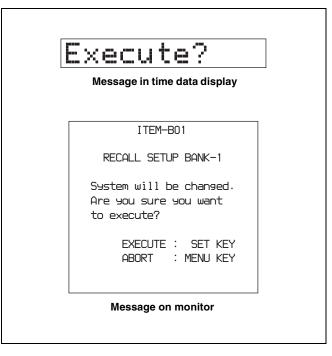
Press the SET button to recall the settings and switch to the line mode saved in the menu bank. When you power the unit off and then on again, it will use the line mode and settings of the selected bank.
