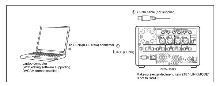
For the method of transferring video/audio signals (AV/C data) to a nonlinear editing system, refer to the manual provided with the editing software to be used.
