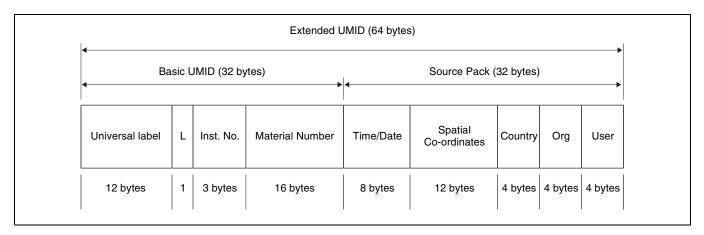
Globally unique ID is automatically recorded in clip units. The Extended UMID is metadata that provides additional information such as location, time/date, company and so on.
