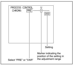
**3** If you selected "VAR" in step **2**, set the parameter value by holding down the corresponding button and rotating the jog dial, while viewing the video.
