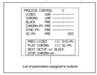
2 Hold down the following buttons and press the RESET button to select "PRE" (PRESET: factory preset setting) or "VAR" (VARIABLE: adjustable setting). Each press of the button switches between "PRE" and "VAR."
