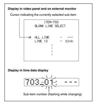
With the SHUTTLE button held down, rotate the jog dial or shuttle dial to change the setting.
