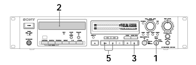
Select the input signal using the INPUT switch on the front panel.
