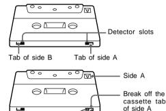
If you later want to reuse the tape for recording, cover the broken tab with adhesive tape. However, be careful not to cover the detector slots which allow the tape deck to automatically detect the type of tape.
