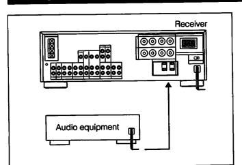
Connect the AC power cord of each piece of equipment to the AC outlet on the receiver so that you can turn the equipment on and off using the receiver's POWER switch.
