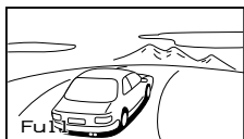
Full An image with an aspect ratio of 4 to 3 enlarged to the left and right edges of the screen.
