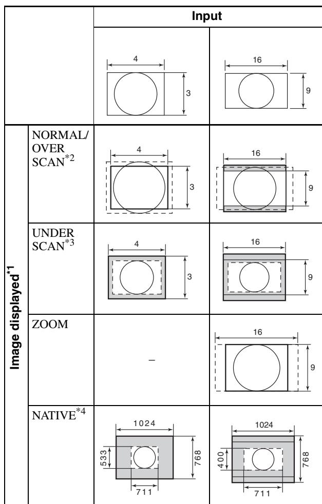
\*1 The image illustrated shows the input signal by broken line and the efficient picture size by the solid line.
