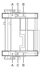
A and C: Sets the stand towards the back. B and C: Sets the stand towards the front.
