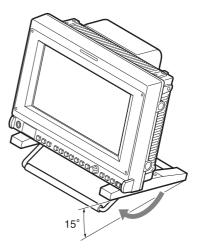
The mounting position of the stand can be changed. Move the mounting screws on the underside of the stand to positions A and C, or positions B and C.
