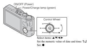
Press the ON/OFF (Power) button. Date & Time setting is displayed when you press the ON/OFF (Power) button for the first time.
