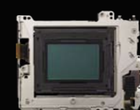
SteadyShot INSIDE unit for 35mm full-frame format sensor
