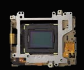
SteadyShot INSIDE unit for APS-C format sensor
