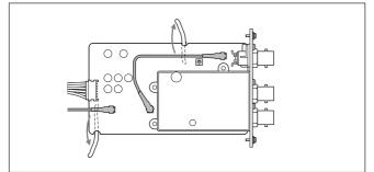
**3** Change the connections for both cables as shown below.
