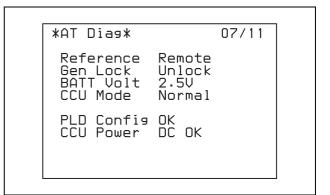
**Reference:** Operation mode of the phase adjustment **Gen Lock:** Locking status
