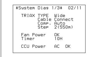
TRIAX TYPE: Type of Triaxial circuit
