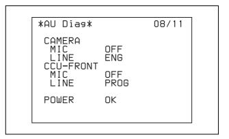
CAMERA MIC: Input status of the camera microphone (on/off) CAMERA LINE: Pathway of the intercom signal of the camera (ENG/PROD/PRIV) CCU FRONT MIC: Input status of the unit's
