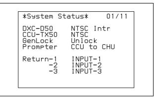
**DXC-D50:** Model name and format of the connected camera
