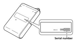
The Passkey is the last 4 digits in the serial number on the back of this unit. Once connection is authorized, you do not need to enter your Passkey again to connect.
