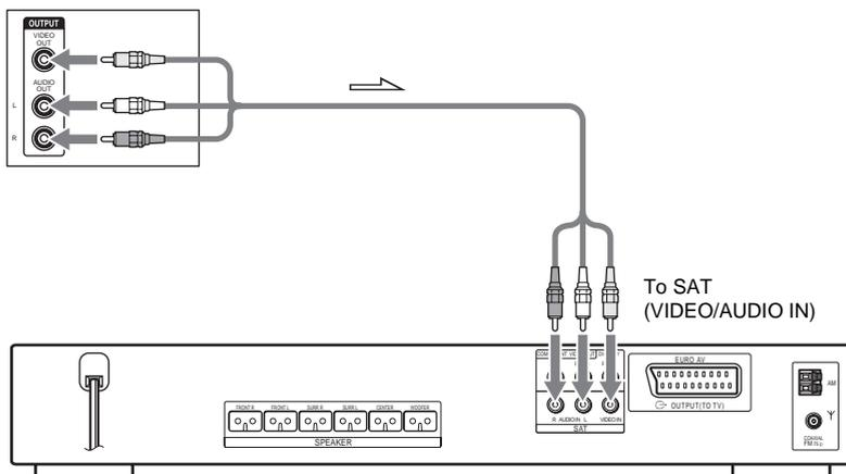
To connect the VIDEO/AUDIO OUT jacks of other component to the SAT (VIDEO/AUDIO IN) jacks of this system
