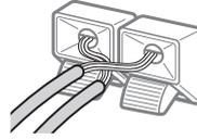
After connecting all the components, speakers, and AC power cord (mains lead), output a test tone to check that all the speakers are connected correctly. For details on outputting a test tone, see page 83. If no sound is heard from a speaker while outputting a test tone, or a test tone is output from a speaker other than the one currently displayed on the Setup Display, the speaker may be short-circuited. If this happens, check the speaker connection again.
