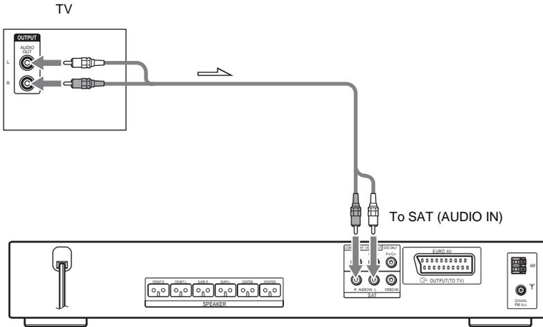
To connect the AUDIO OUT jacks of a TV to the SAT (AUDIO IN) jacks of this system
