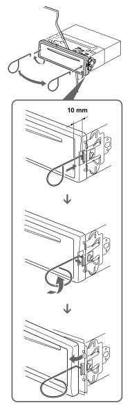
2 Insert a flathead screwdriver between the bracket and mounting spring. Gently pry the spring toward the unit while pulling the unit out a little. Repeat on the opposite side and remove the unit.
